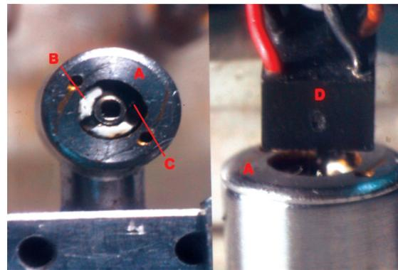
**Figure 4.** Composite view of the posterior aspect of the head of the handpiece and the optical tachometer. Turbine motor was painted half white and half black to facilitate tachometer reading. Posterior aspect of the handpiece (a); white half of turbine rotor (b); black half of turbine rotor (c); and optical tachometer (d).
