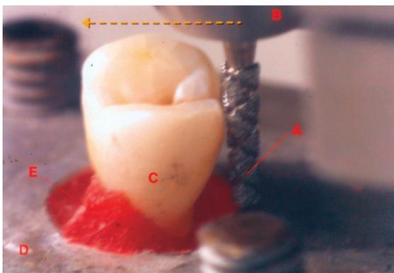
**Figure 6.** Close-up view of cutting action. Coolant spray was always directed to the bur without interference. TDA bur (a); handpiece head (b); premolar tooth (c); stainless steel supporting plate (d); and autopolymerizing pattern resins (e). Arrow indicates direction of cutting action.
