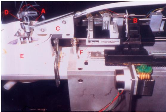
**Figure 5.** General view of system set up. High-speed handpiece (a); handpiece tubing (b); handpiece mount (c); optical tachometer (d); custom-made water bath (e); and low-friction ball bearing slider (f).
